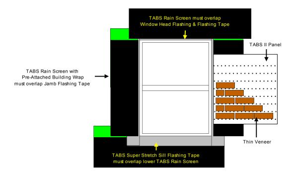
Note: When installing Tabs Rain Screen Panel, always install panels hand tight panel to panel.
